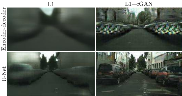
Figure 4: Adding skip connections to an encoder-decoder to create a “U-Net” results in much higher quality results.
